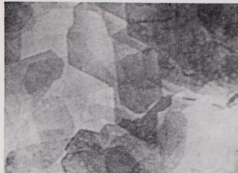
Phot. 1. Electron micrograph of polycrystalline aggregates of kaolinite from Jegłowa (sample S-0 ). Magn. \times 98\ 000
