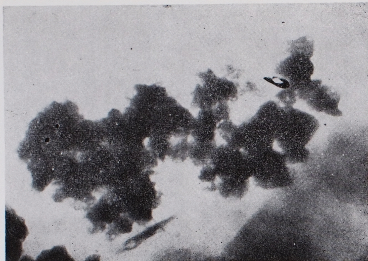
Phot. 3. Electron micrograph of kaolinite aggregates after treating with 4 n NaOH during 25 h (sample S-1). Magn. \times 33\ 000
